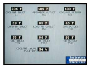
The ICHM controller communicates with the generator controller and operates all on-board equipment and the cooling tower. The ICHM provides a single connection to the engine controller which will provide data acquisition, operation control and status indication. Local status indication and alarm contacts are also provided. The ICHM power panel distributes power to the various electrical components and the cooling tower.
